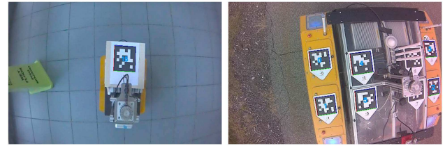
Fig. 5. Detected AprilTag mounted on the ground robots captured from one aerial robot’s downward-facing camera.
