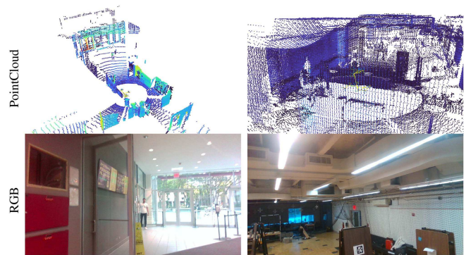
Fig. 3. Indoor-NYUARPL environment. Pointcloud data (top row) is captured by the ground robots, and the color images (bottom row) are captured by the aerial robots. Each column shows one subgroup of one aerial robot and one ground robot exploring different parts of the environment.
