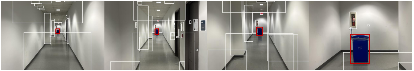
Fig. 5: Demonstrating our system’s ability to detect, track, and navigate toward an asymmetrically shaped trash can within a featureless narrow corridor, hence highlighting the efficacy of our visual control method.
