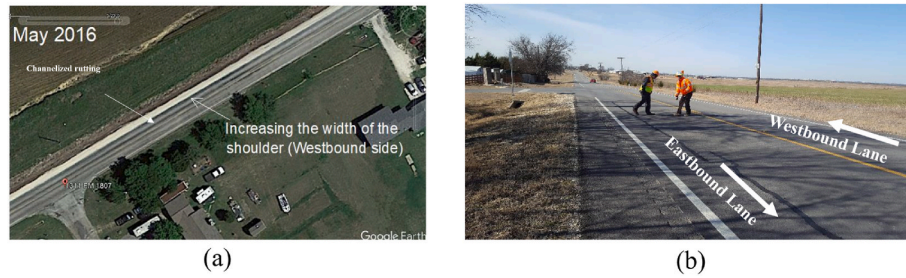
Fig. 2. Pavement distresses on FM 1807: a) channelized rutting observed during May 2016, b) longitudinal cracks observed after six months of the major rehabilitation work during January 2018.
