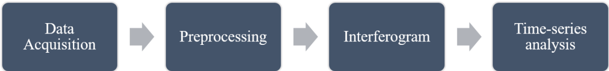
Figure 4. Typical processing steps for time-series InSAR
