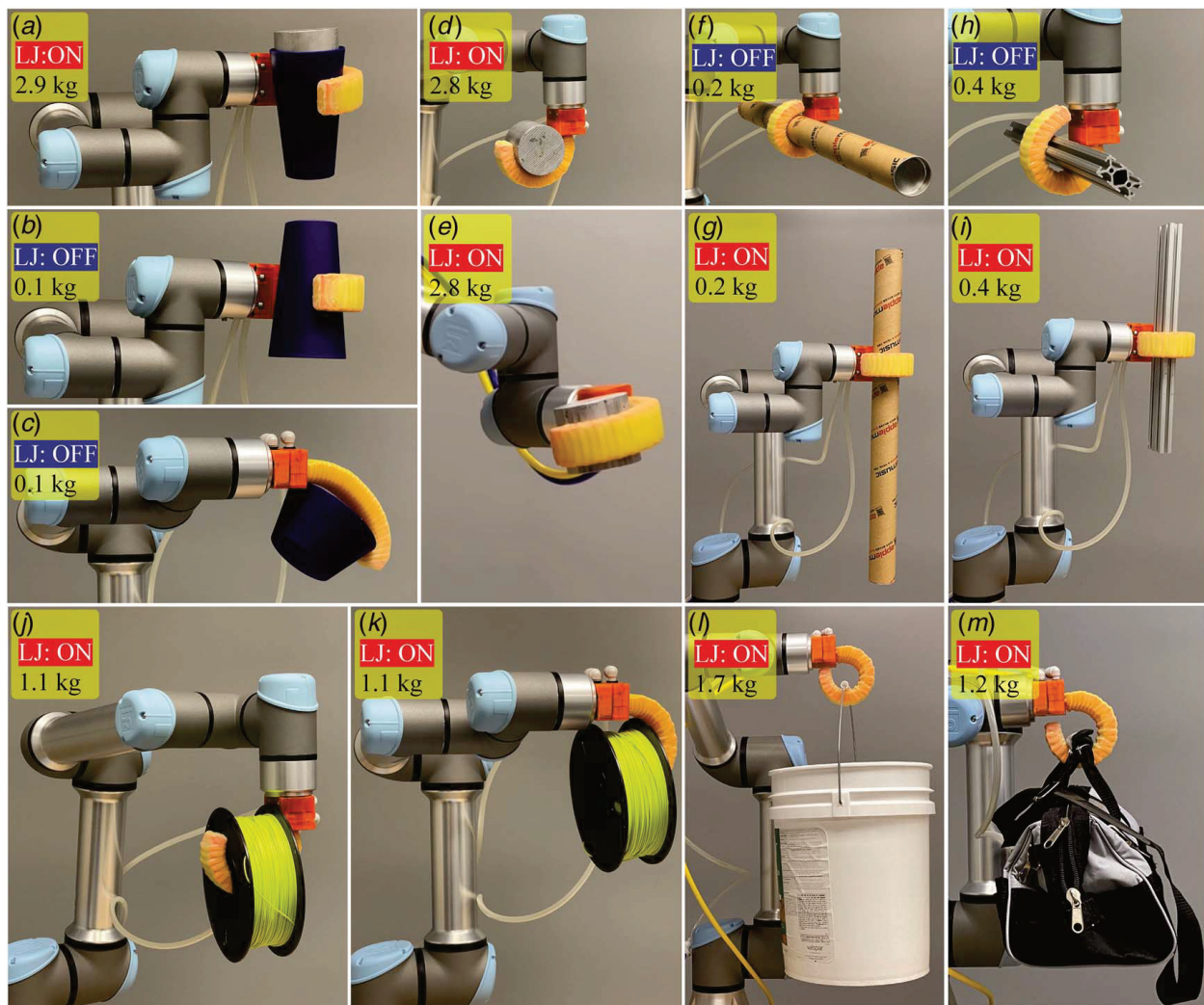
Fig. 7 Selected demonstrations showing the high adaptation feature of the gripper (LJ stands for layer jamming, ON and OFF indicate the actuation status of layer jamming)
