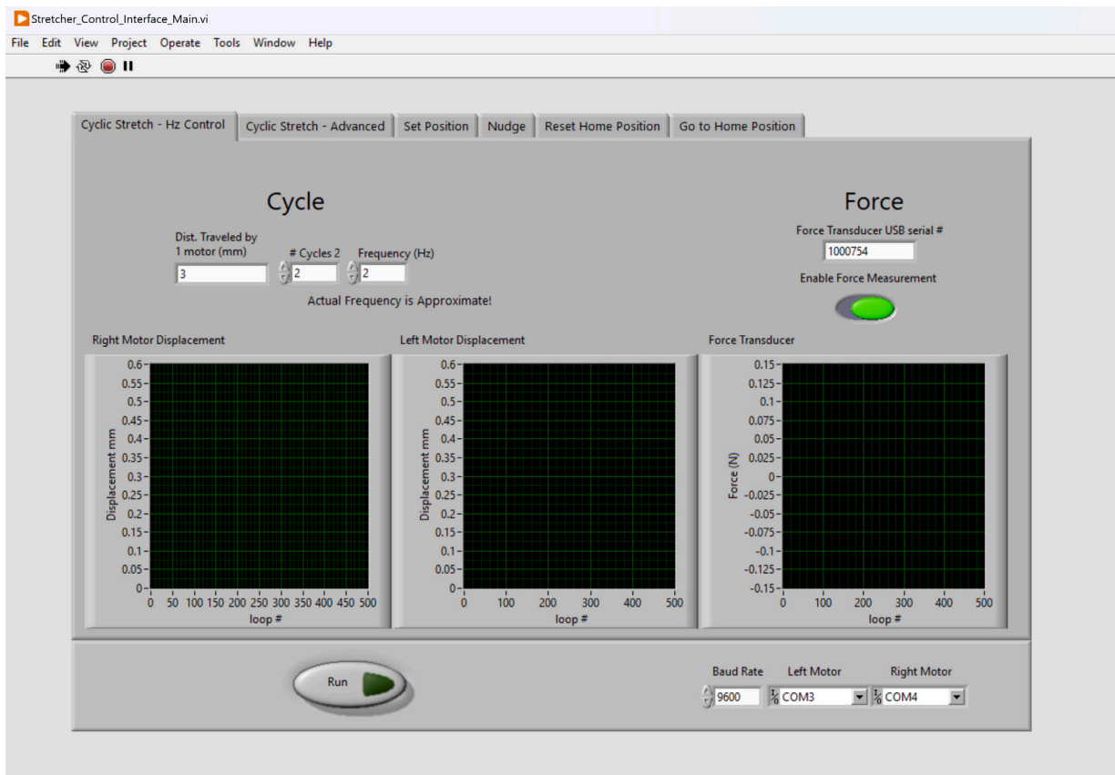
Fig. 6. The Cyclic Stretch-Hz control can be used for cyclic tensile testing as a simpler alternative to the advanced tab, utilizing frequency (Hz) instead of velocity (mm/s).
