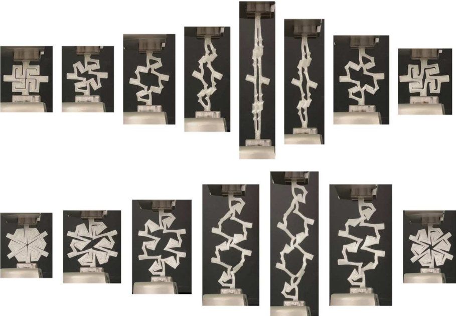
Fig. C6. Changes in the microstructure of TPU square (top) and hexagon (bottom) kerf cell during loading-unloading
