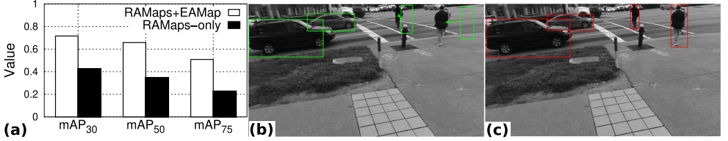
Fig. 13. (a) mAP comparison between RAMaps-only and RAMaps+EAMap model under the IoU threshold of 0.30, 0.50, and 0.75. (b) Predictions of RAMaps-only model. (c) Predicted bounding boxes of RAMaps+EAMap model.
