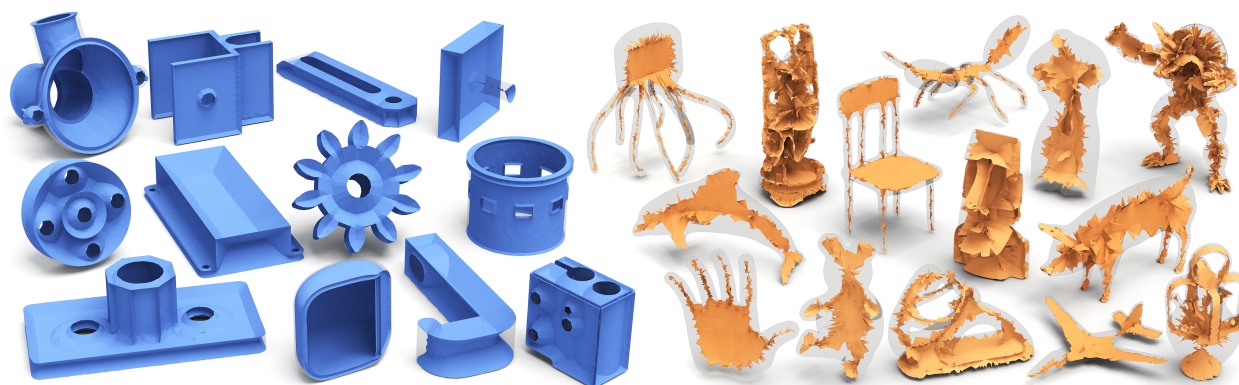
Fig. 1. A gallery of our topology-preserving 3D medial axis results. The input shapes are shown in transparency, while the computed medial axis are shown in blue (left) and brown (right) colors. The left side displays the medial axis computed on CAD models, and the right side shows those on organic models.
