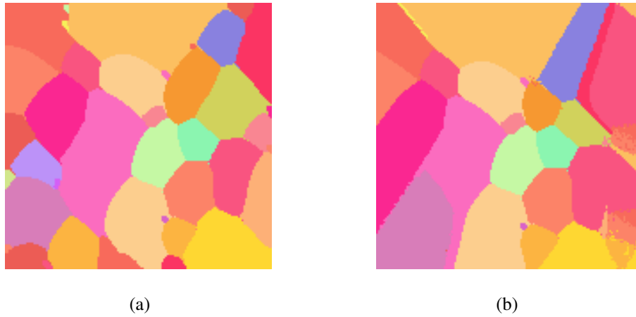
Fig. 8 (a) Cropped section of the color corrected image used in MRF reconstruction, (b) Reconstruction of the image with a window size of 29 and a resolution of 150 \times 150 pixels.
