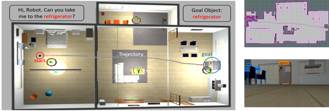
Fig. 5: ROS Gazebo simulation: a home environment. The robot receives voice input from the commander to navigate to the desired object. The home environment (left) with visualization of the navigation map (right top) and onboard camera view with objection detection (right bottom).
