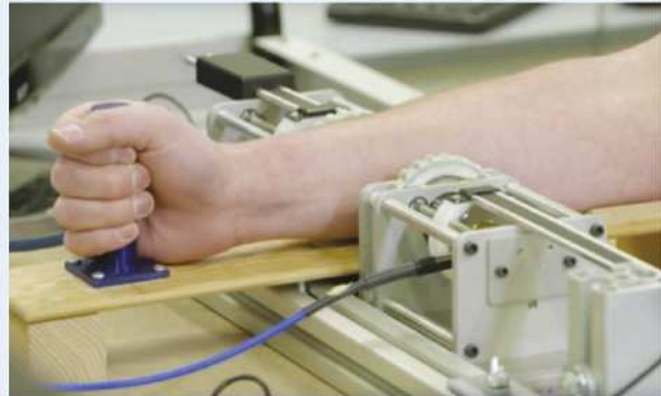
FIGURE 8. A microwave transmission measurement system for hydration-level evaluation. The antennas are in contact with the skin at the midpoint of the forearm. (Source: Garrett et al. in the graphical abstract of [71].)
