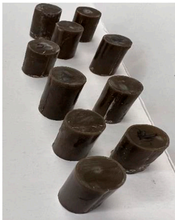
Figure 1. Synthesized vitrimer regolith composite samples.
