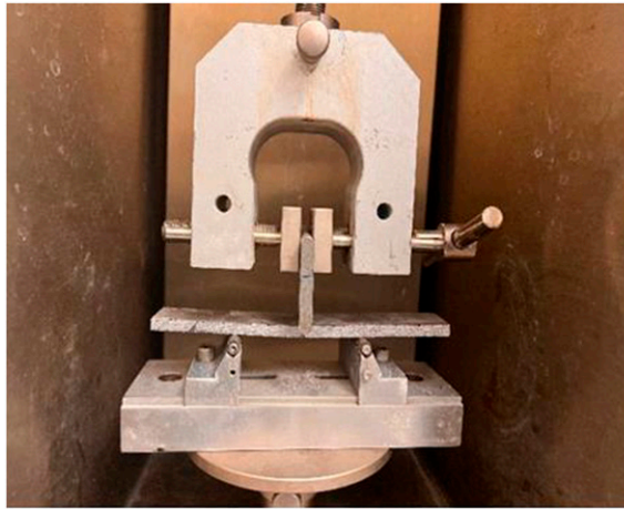
Figure 7. Glass fabric reinforced SMV and SMV-regolith laminated composites under a three-point bending test.
