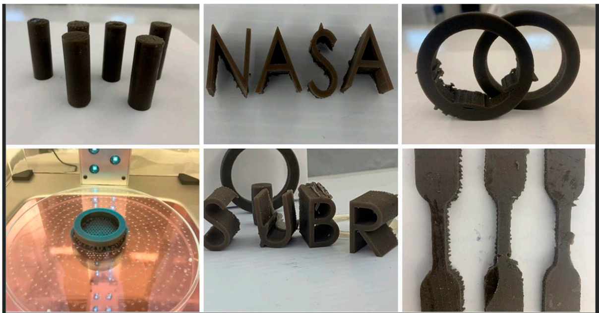
Figure 8. 3D printed SMV-regolith composite samples using LCD printer.
