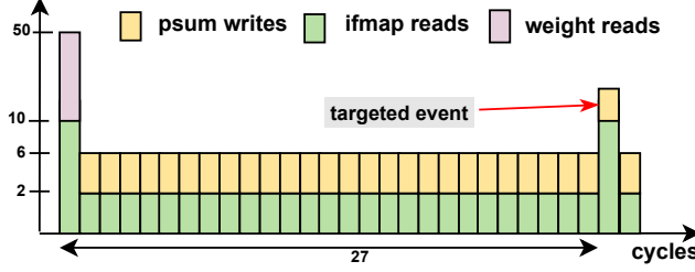
Fig. 7. Cycle-wise number of data reads/writes until the targeted event of Alexnet Conv2 layer in WS(12,4).
