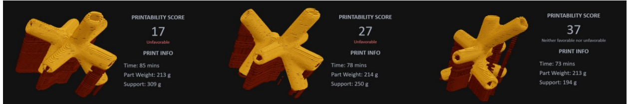
Figure 4: Showing three different build orientations of D3 and the manufacturability outcomes calculated using the Cura slicing engine and Equation 1 for each orientation
