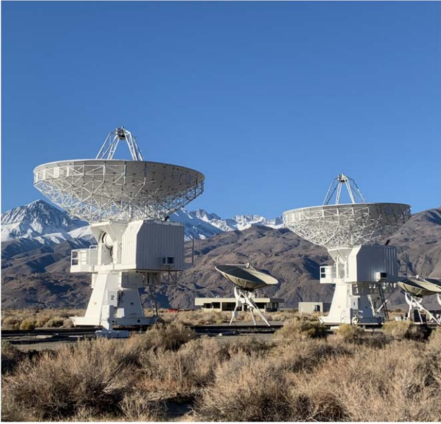
Figure 1. The two 10.4 m Leighton antennas, located at OVRO, that are used for the initial SPRITely deployment. The receivers are housed within the sidecabs at the Nasmyth focus of each antenna, located nearer to the viewer. The smaller dishes are part of the 110-antenna Deep Synoptic Array. In the background is the Mayer control building, which houses the final steps of the signal processing chain and the data processing computers for the telescopes.
