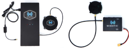
Fig. 2. The WiBotic transmitter (left) and onboard charger and receiver (right), along with their corresponding antenna. Figure adapted from [6].
