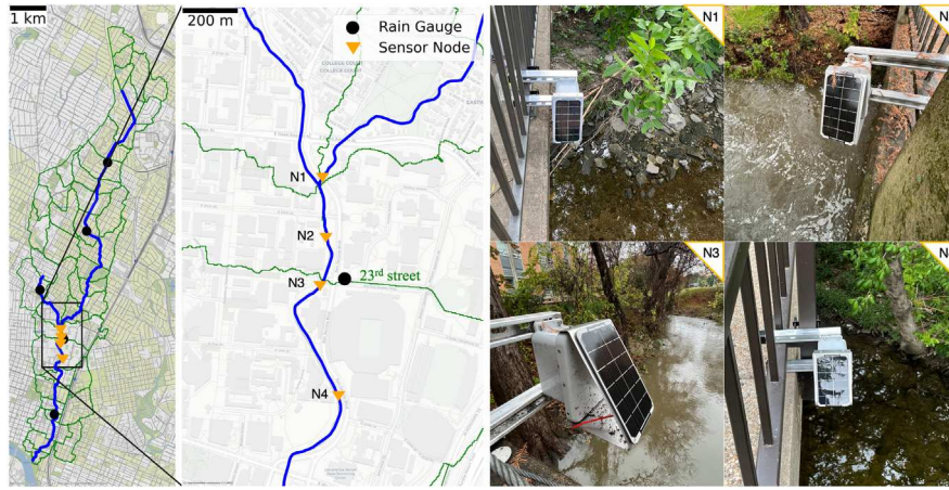
Fig. 3. Map and photos of wireless sensor network in Waller Creek watershed.
