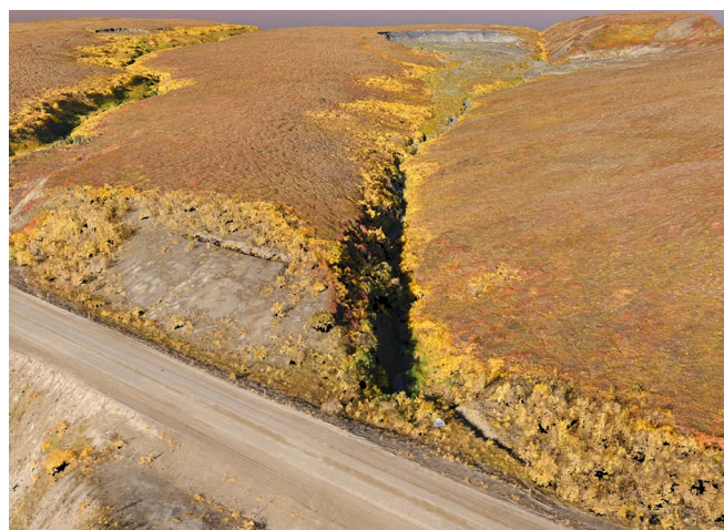
FIGURE 11 | Inset from a three-dimensional fly-through video (Supporting S1) of a photogrammetric survey by drone, capturing retrogressive thaw slumps at NT km 28.5, Dempster Highway, Canada. The video shows the position of the slump with respect to the highway, the potential threat that downslope debris flows pose to the highway, the debris that has infilled the valley, and how the main slump has caused multiple secondary slumps by undercutting the opposing slope. Photograph and video by Jurjen van der Sluijs, 2022. [Colour figure can be viewed at wileyonlinelibrary.com ]
