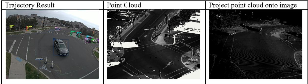
185 **Figure 5:** Tracking and trajectory results, 3D Point Cloud, Projected point cloud image
