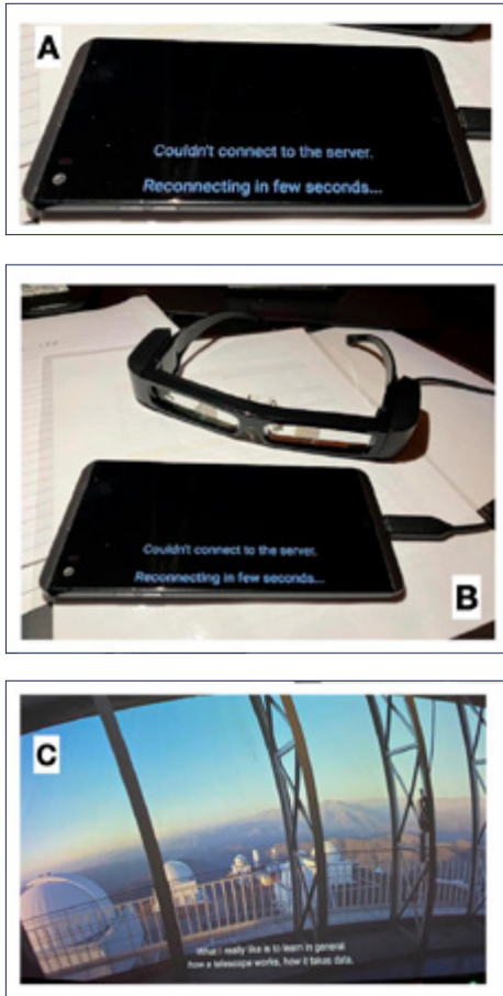
Figure 1: A) Handheld device (LG Phone); B) AR glasses (Epson Moverio BT-30C supported by LG phone) C) On-Screen Captions.
