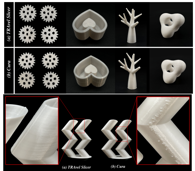
Figure 21: Top: All models printed in PLA with (a) TRavel Slicer, (b) Cura. Bottom: Zoomed in views of the seams generated by each toolpath.
