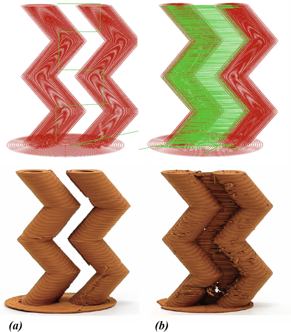
Figure 17: Test: Vertical Nesting. A model with two zig-zagging pillars sliced with TRaVel Slicer (a) and Cura (b). The top images show toolpath visualizations. Red: extrude paths, green: travel paths.
