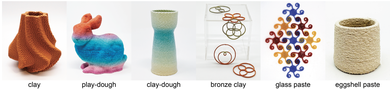
Figure 2: We 3D print a variety of clay-like materials that vary drastically in their properties, aesthetics, and affordances.
