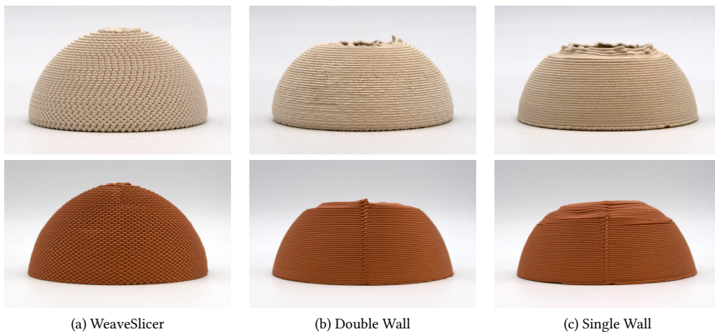
Figure 15: Fired half Spheres printed with (a) WeaveSlicer, (b) double wall, and (c) single wall toolpaths, N = 3 . The top row was printed with the Eazao printer and the half spheres have a 7.5cm diameter. The bottom row was printed with the 3DPotter printer and the half spheres have a 15cm diameter.
