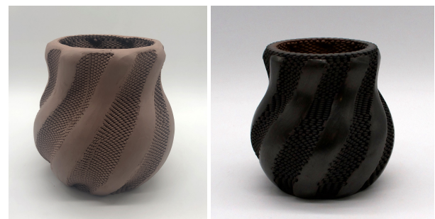
Figure 20: Anfractuuous Transmutation made by Resident 2 and sliced with WeaveSlicer. It is unfired on the left, and finished by pitfiring on the right. Resident 2 smoothed certain areas of the pot and left the texture of the WeaveSlicer toolpath in others.
