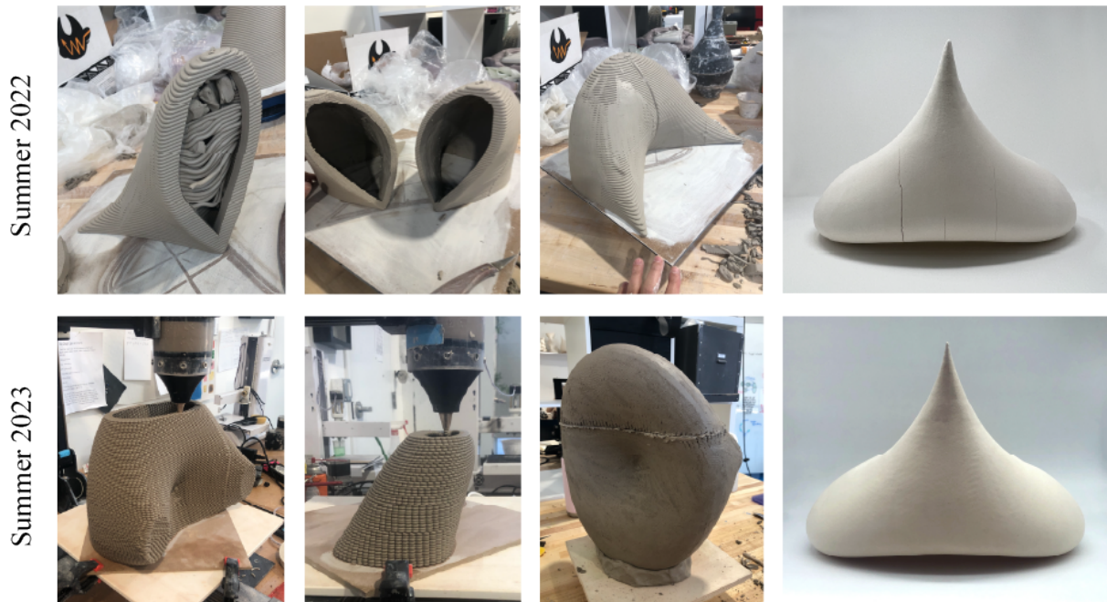
Figure 18: Top: Workflow of Horned Torus build from summer 2022 residency from left to right. One piece with infill of a four-part sculpture immediately after printing. Infill is removed from each piece. The pieces are smoothed and joined together to create one half of the final piece. Multiple cracks developed along print lines after firing. Bottom: Workflow of Horned Torus build from summer 2023 residency from left to right. Large part of the body of the sculpture without any infill. Smaller part of the body of the sculpture without any infill. The two pieces are smoothed and joined together. No cracks appeared after firing.
