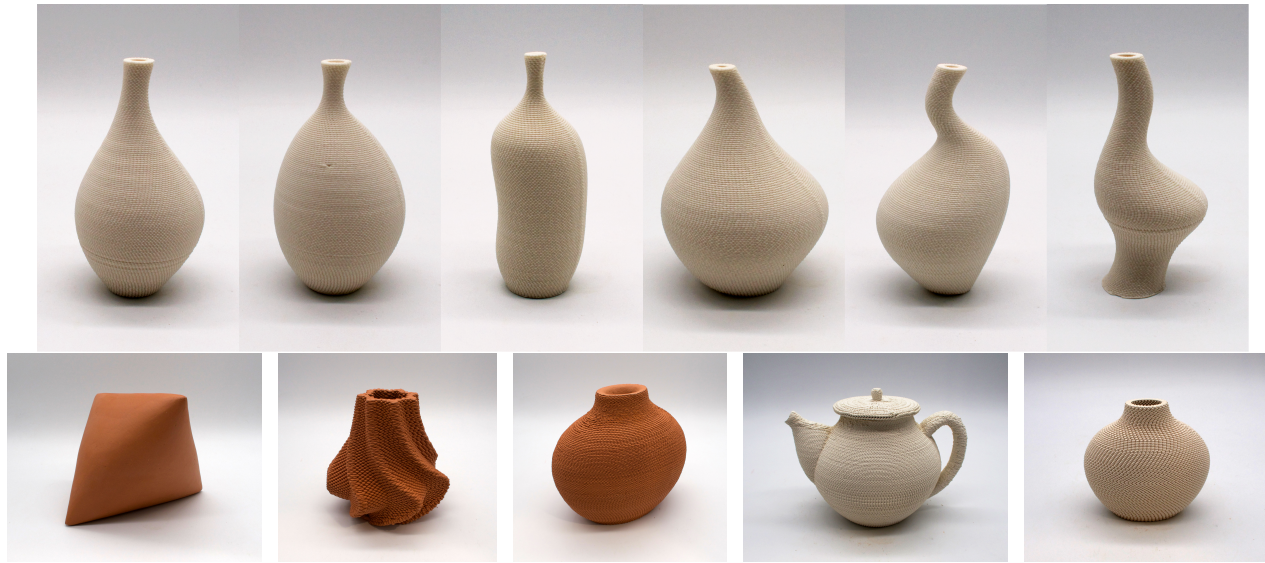
Figure 21: Additional artifacts printed using WeaveSlicer. Top: Porcelain vases printed on the Eazao Zero printer with a nozzle width of 1.5mm. Bottom (left to right): Earthenware sculpture printed in two parts using WeaveSlicer, earthenware vessel printed with WeaveSlicer on the 3D PotterBot 10 PRO with a 3mm nozzle, earthenware vessel printed with WeaveSlicer on the 3D PotterBot 10 PRO with a 3mm nozzle, porcelain teapot printed on the Eazao Zero printer with a nozzle width of 1.5mm, stoneware vessel printed on the Eazao Zero printer with a nozzle width of 1.5mm
