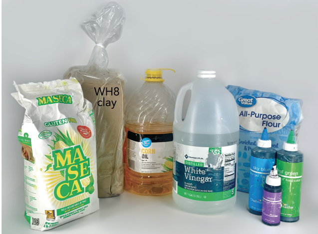
Figure 4: Ingredients used to make clay-dough from left to right: corn flour, WH8 stoneware clay, vegetable oil, vinegar, wheat flour, food dye, and (not pictured) water.
