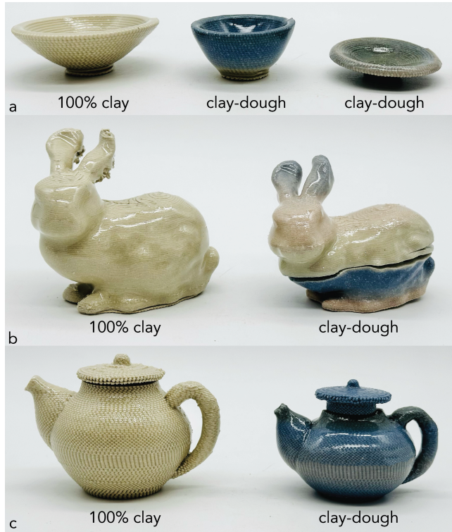
Figure 14: (a) Bowl, (b) Stanford Bunny, and (c) Teapot forms printed in 100% clay and printed in a random pattern of clay-dough.
