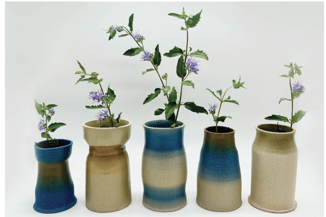
Figure 2: Forms created through our material-oriented approach with clay-dough that started as identical 3D printed cylinders and then shrunk into differently shaped vessels when fired.
