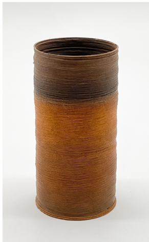
Figure 17: A sintered/fired print that combines bronze (bottom 3/4) and clay (top 1/4) in a single print.
