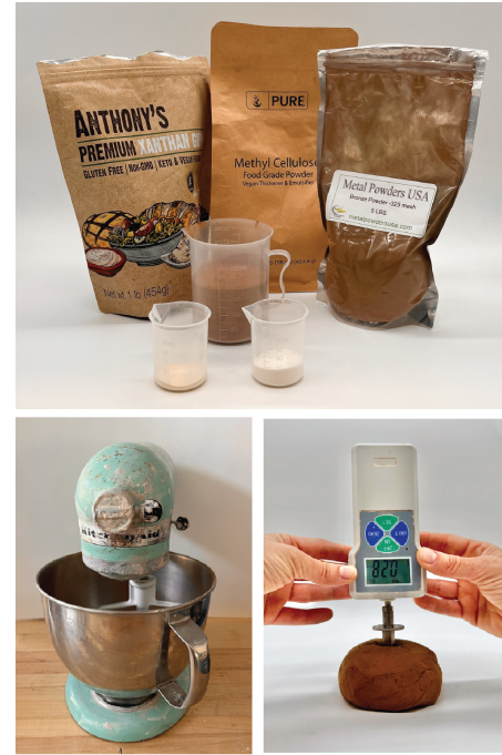
Figure 2: Recipe ingredients (top). Mixing ingredients in a kitchen mixer to form a uniform material with a clay-like consistency (bottom left). Measuring the indentation hardness of the metal clay (bottom right).
