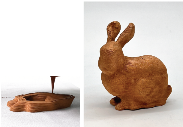
Figure 16: A Stanford bunny during printing (left) and after sintering and cleaning (right).
