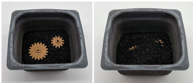
Figure 7: Parts are buried in activated carbon before firing.
