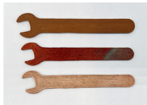
Figure 8: Three wrenches, from top to bottom: after printing, after firing, and after cleaning
