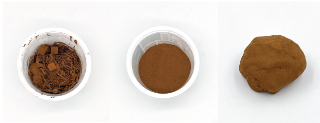
Figure 3: Process for recycling un-sintered bronze clay. Print waste is collected (left), ground back into powder using a blender (center), and then mixed with water to form a recycled clay (right).
