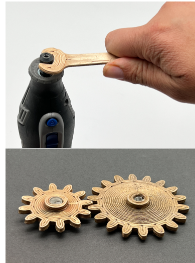
Figure 13: Top: using a 3D printed wrench on a Dremel tool. Bottom: two gears driven by a stepper motor.
