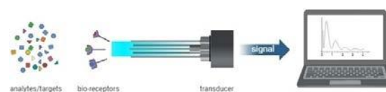
Figure 1. Biosensor Structure. Created with BioRender.com.
