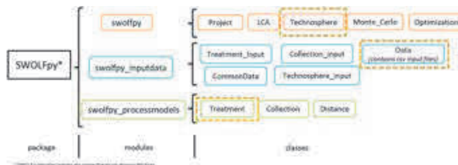
Fig. 1. An extract of SwolfPy classes, highlighting the classes that are modified in the extension proposed. Based on Sardarmehni et al. (2022).
