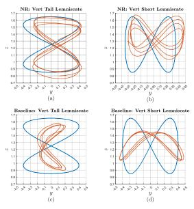
**Fig. 5.** Comparison of Newton-Raphson controller (top row) and Baseline controller (bottom row) on fast vertical lemniscate trajectories with period 3.14 seconds. The Newton-Raphson controller approximately maintains the lemniscate shape, while the baseline controller tracks poorly.
