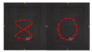
**Fig. 1.** Frames from overhead videos of a quadrotor performing lemniscates and circles using the proposed Newton-Raphson flow controller with the trajectories overlaid.
