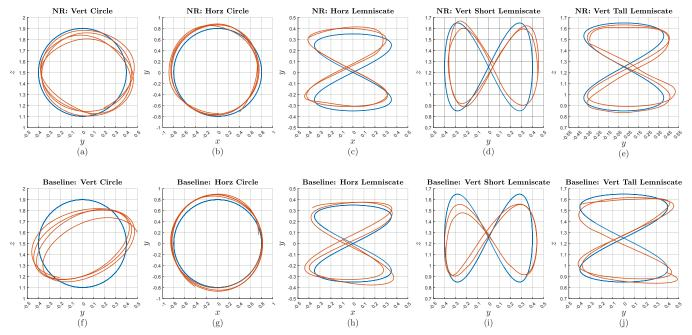
**Fig. 2.** Comparison of five flight trajectories (red) with the reference trajectories (blue). Top row shows results using the Newton-Raphson flow control and the bottom row shows results using the baseline PX4 controller. Axes units are meters. The periods of circular and lemniscate trajectories are 3.14 and 6.28 seconds, respectively. In all cases, the Newton-Raphson flow controller outperforms the baseline controller, evaluated with the root-mean-square error, as reported in Table I.
