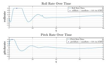
**Fig. 4.** Roll and Pitch Rates Subject to Safety Constraints via Integral CBFs. The rates can be seen to be smoothly limited to a maximum absolute value of  $0.8 \,\mathrm{rad/s}$ .
