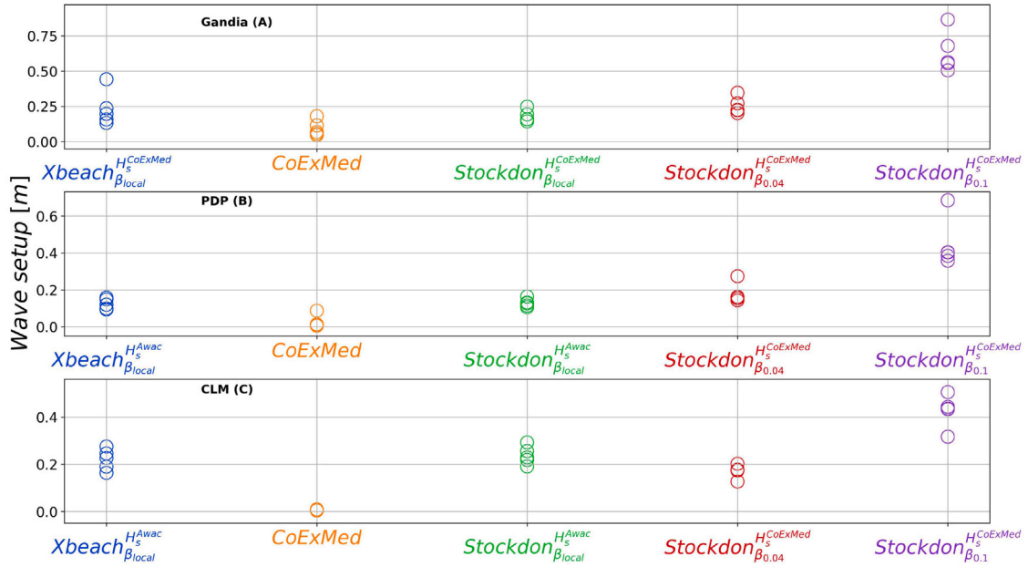
Fig. 4. Wave setup levels of 5 independent events (see Section 4) that occurred between 2012 to 2017 for each study case, at the beaches of Gandia (A), PDP (B) and CLM (C). From left to right, wave setup values from wave_{setup}^{Xbeach} , wave_{setup}^{CoExMed} , wave_{setup}^{\beta_{local}} , wave_{setup}^{\beta_{0.04}} and wave_{setup}^{\beta_{0.1}} .
