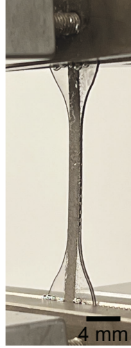
Fig. S6 | Photography of the physical characterization experiments under tensile loading.
