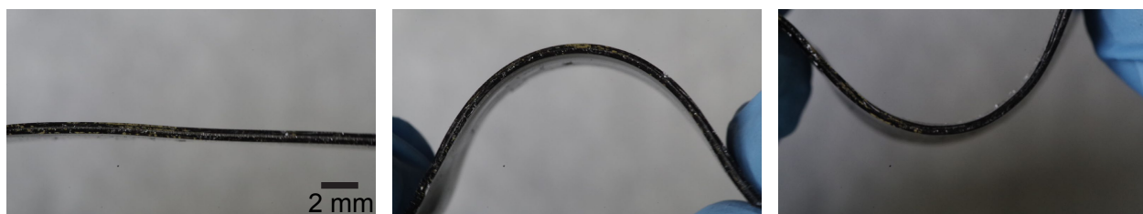
Fig. S19 | Close up photography of bonded circuit under mechanical deformation.
