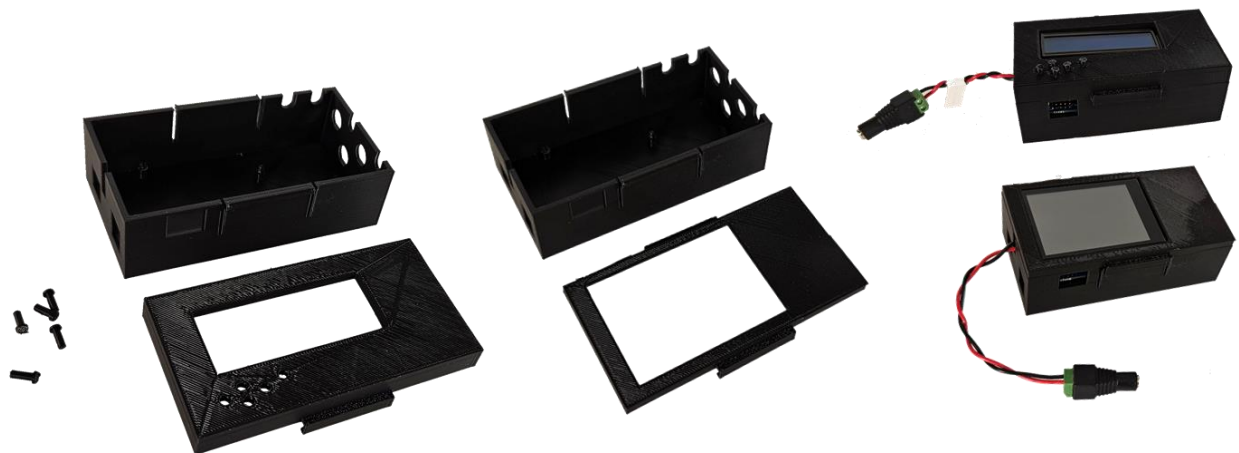
Fig. 6. Pictures of the enclosure for a controller in parts (left) and assembled (right).
