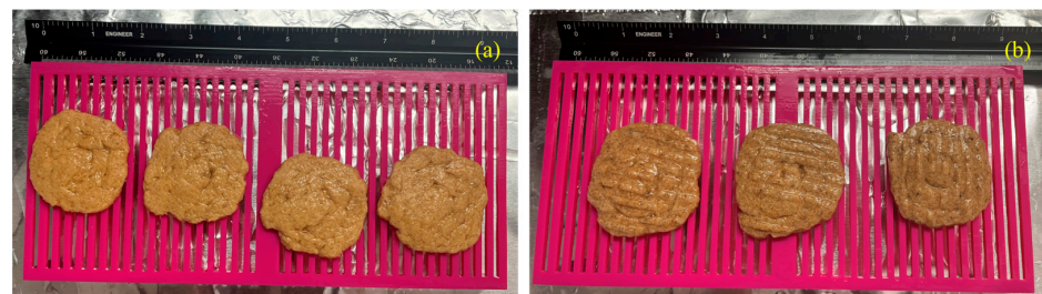
Figure 4. Samples after soaking in crosslinking solution: (a) hemp hurd samples, (b) beechwood sawdust samples.
