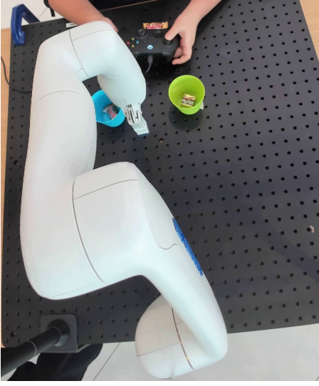
Figure 7: Overhead view of robot in the claw game interaction. A user controlled a Kinova Gen3 Lite robot to pick up one of two cups, despite “assistance” that drove them away from the cup locations.
