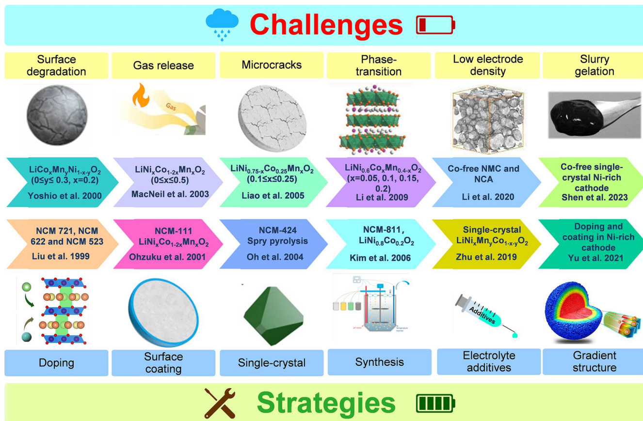
Fig. 2. Schematic illustration of the major challenges and strategies of Ni-rich cathode materials in different stages from crystal structure to practical applications [30–34].
