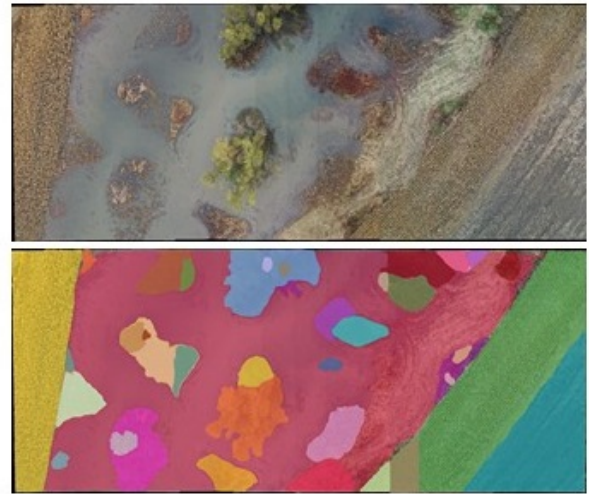
Fig. 4: An example of SAM segmentation result (bottom) on a drone image (top).
