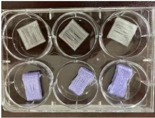
Figure 5. 3DMF Culture Stability. A long-term stability assessment was done based on the ASTM1635 standard for 16 weeks to determine that the base filament wound fibers of 3DMF implants had maintained hydrated stability via the collagen 'resin' alone. FFF (top) and 3DMF implants retained their shape and structure, shown here, air-dried after 4 months of hydration, with samples used for assessing degradation by mass loss (table 1 below) and subsequent for long-term tensile testing to determine strength retention.
