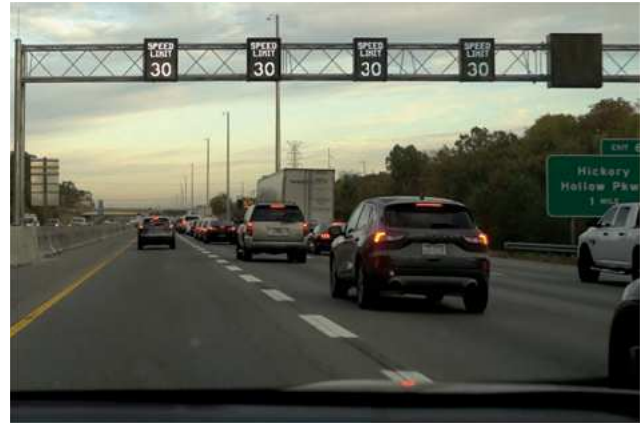
Fig. 1. Recurring Dilemma: Variable Speed Limit (VSL) gantry shows a 30 mph speed limit on Interstate-24. Prevailing traffic is shown to regularly exceed the VSL by a large margin. In this work we demonstrate an automated vehicle controller that follows the VSL on the gantry when nearby vehicles do, and adopts a higher speed when prevailing traffic is moving much faster than the posted speed.
