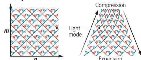
Laser pulses from the short (red) and long (blue) loops are observed as a function of the number of round trips ( $m$ , spatial variable) and the number of accumulated time differences ( $n$ , time variable). Varying the coupling between loops slowly creates isentropic compression or expansion by bringing the lattice mode sites closer or further apart.
