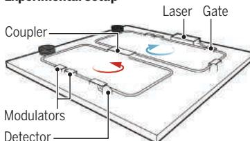
Two coupled fiberoptic loops (red and blue) that have slightly different lengths create a timing difference. A laser injects light pulses that then split into the two loops through a coupler. Light amplitude and phase can be modulated along the loops.
