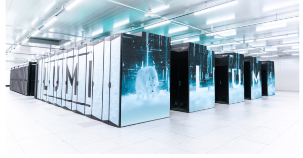
Fig. 1. LUMI, EURO HPC's pre-exascale system with AMD mi250x GPU-accelerated nodes. Each GPU node consists of the four AMD mi250x GPUs, each of which has two graphics compute dies (GCDs) being individual Heterogeneous-Compute Interface for Portability (HIP)-programmable devices. Photo copyright Fade Creative.
