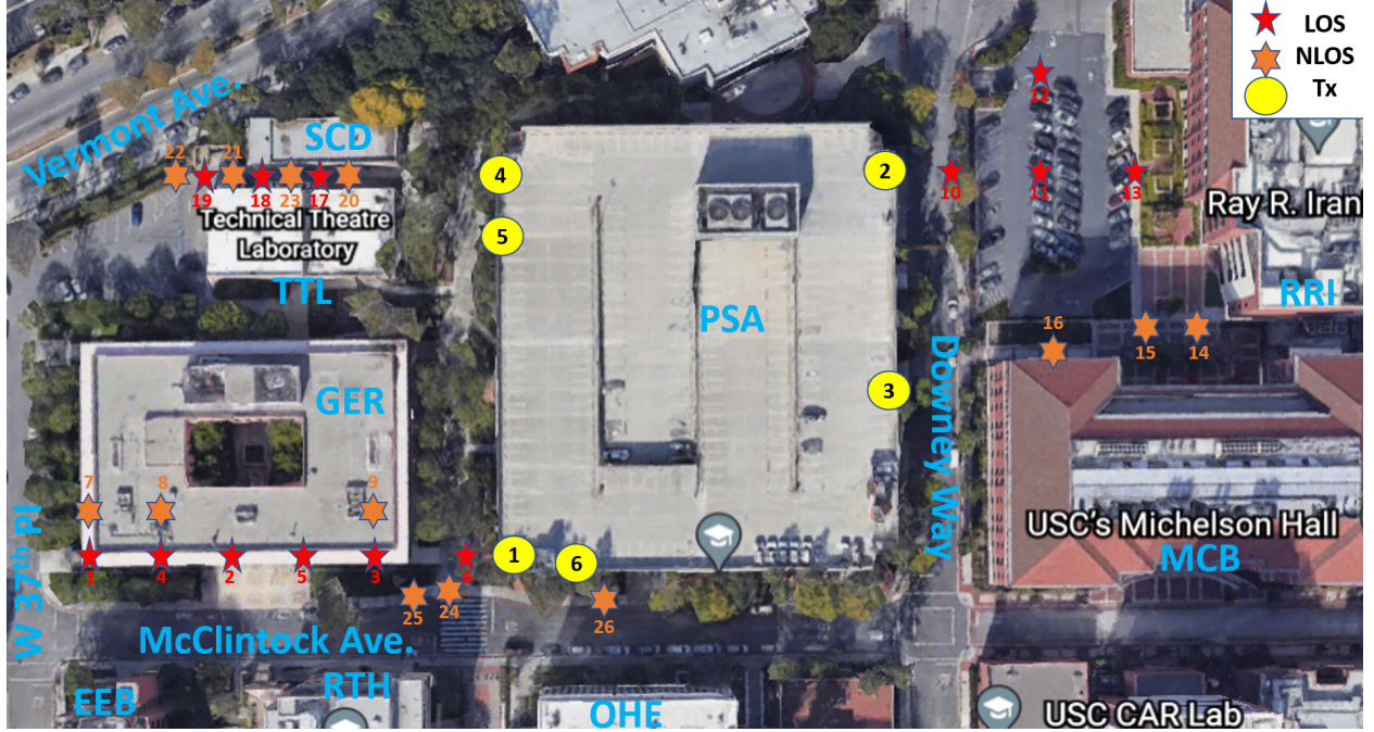
Fig. 2: Microcellular campaign measurement scenario.
