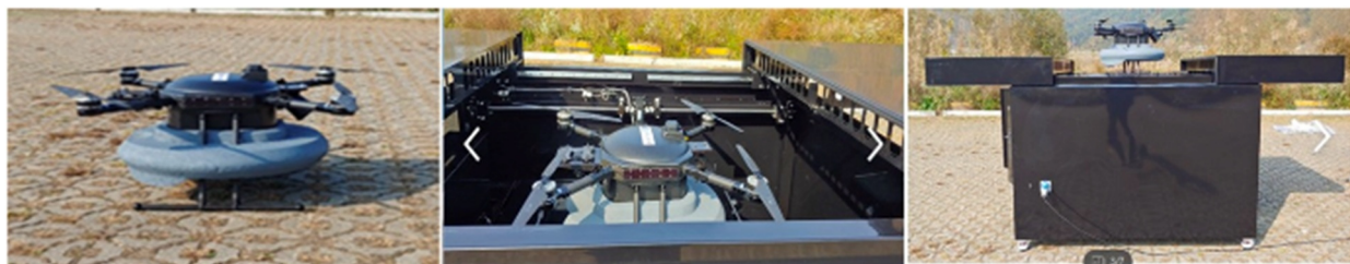
FIGURE 17 Development of a drone and station system for monitoring dams and rivers. 228
