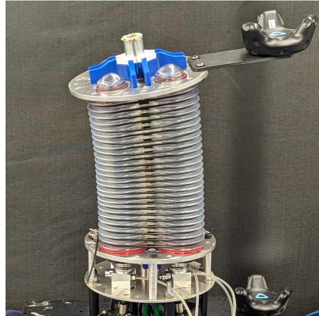
Fig. 1. Graphic of the continuum joint used in this paper, referred to as the “grub”. The grub has four pneumatically-actuated plastic chambers that control its motion. Angle position and velocity states are estimated using two HTC Vive trackers.
