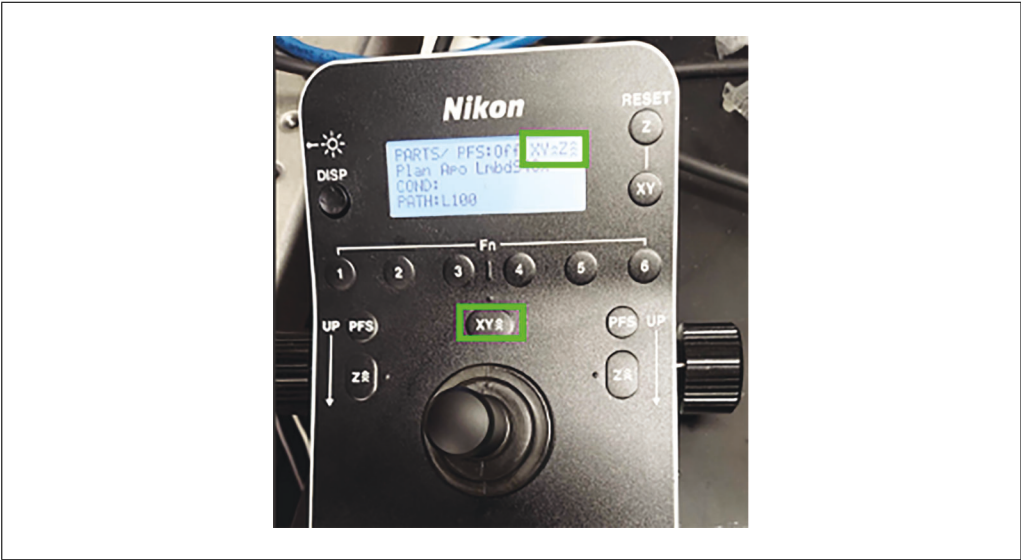
Figure 2 Nikon joystick control box with XY speed lowered to 2 arrows. Control box showing adjusted XY speed to decrease risk of oil droplet displacement.
