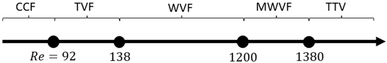
Fig. 4—Flow regime in a single-phase TC flow (Yoshida et al. 2009).
