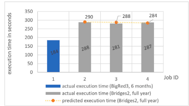
Fig. 12. Demonstration of execution time prediction with LaunchAgent . Job 1 is a half-year DHSVM execution on BigRed3, and job 2,3,4 are full-year DHSVM execution on Bridges2.
