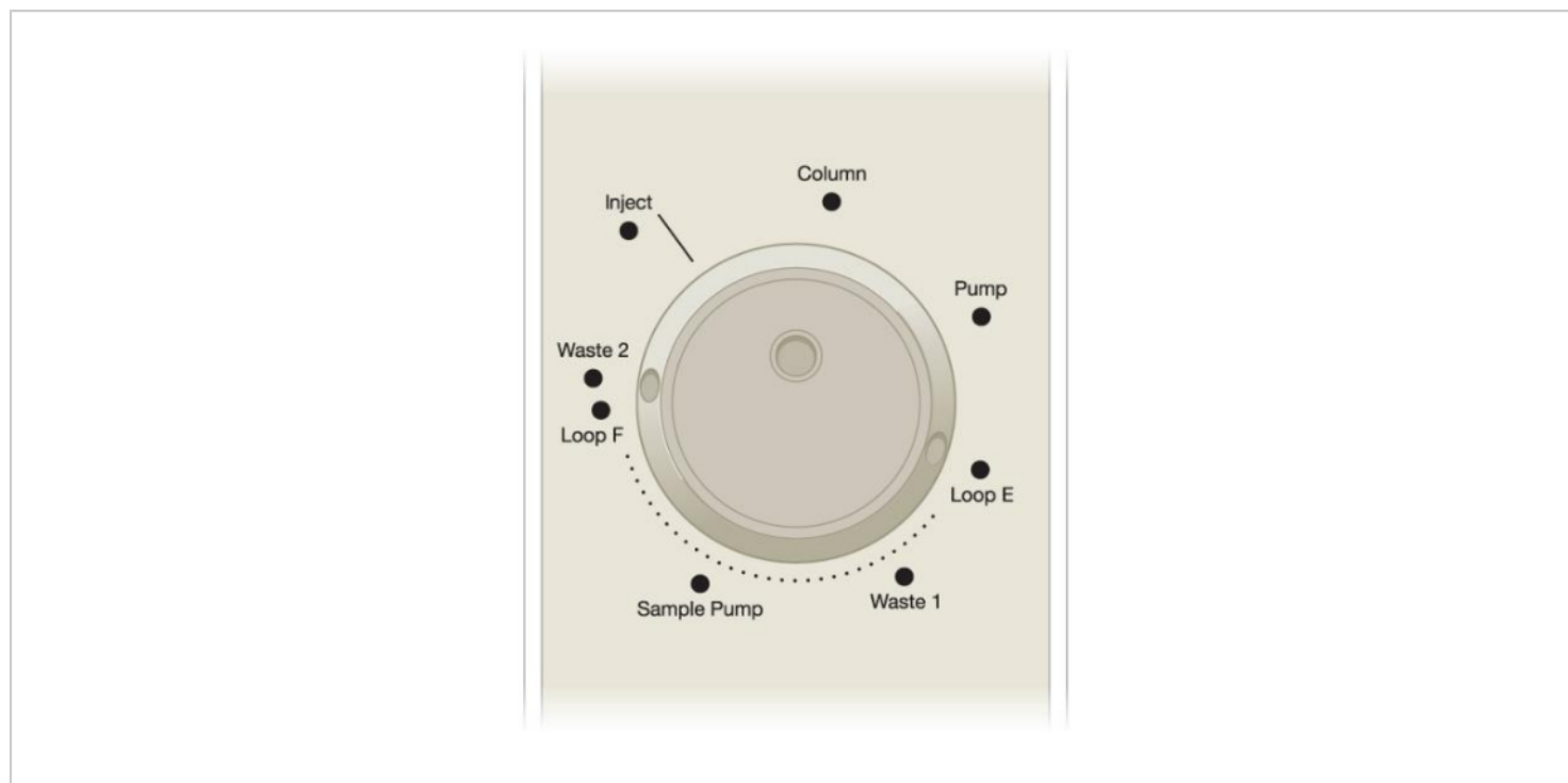
Figure 3: Injection module of the Fast protein liquid chromatography system. The various ports of the injection module connect the fast protein liquid chromatography system to the column, sample loop, and waste. The image was taken with permission from 10 . Please click here to view a larger version of this figure.
