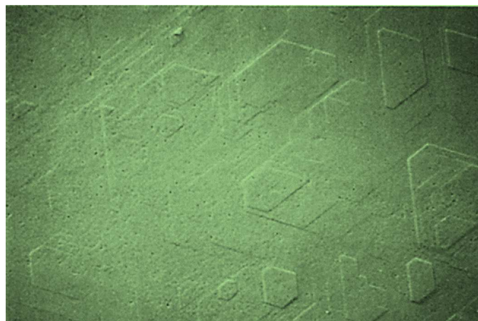
Fig. 9. SEM photographs of (111) Si epitaxy layers grown at 4 mA/cm 2 . (Adapted with permission from J. Electrochem. Soc., 123 (1976) 381–383.).
