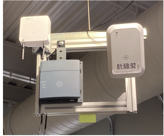
Figure 4. An example of three of four antennas mounted to a frame in CVAC. Only one system was powered on at a time unless specified.
