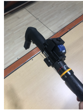
Figure 5. An example of the AFCS tool, with an RTLS tag affixed.
