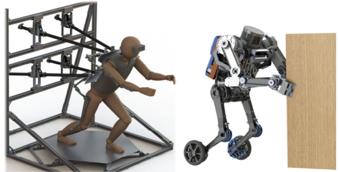
Fig. 1. The vision of SATYRR performing Dynamic Mobile Manipulation via teleoperation with the Human Machine Interface.
